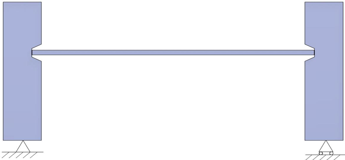
**Figure 6: Experimental Model of Simply Supported Beam**
